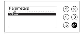
By using the UP and DOWN keys it is possible to select the set-point to modify: SC1 summer set-point.
