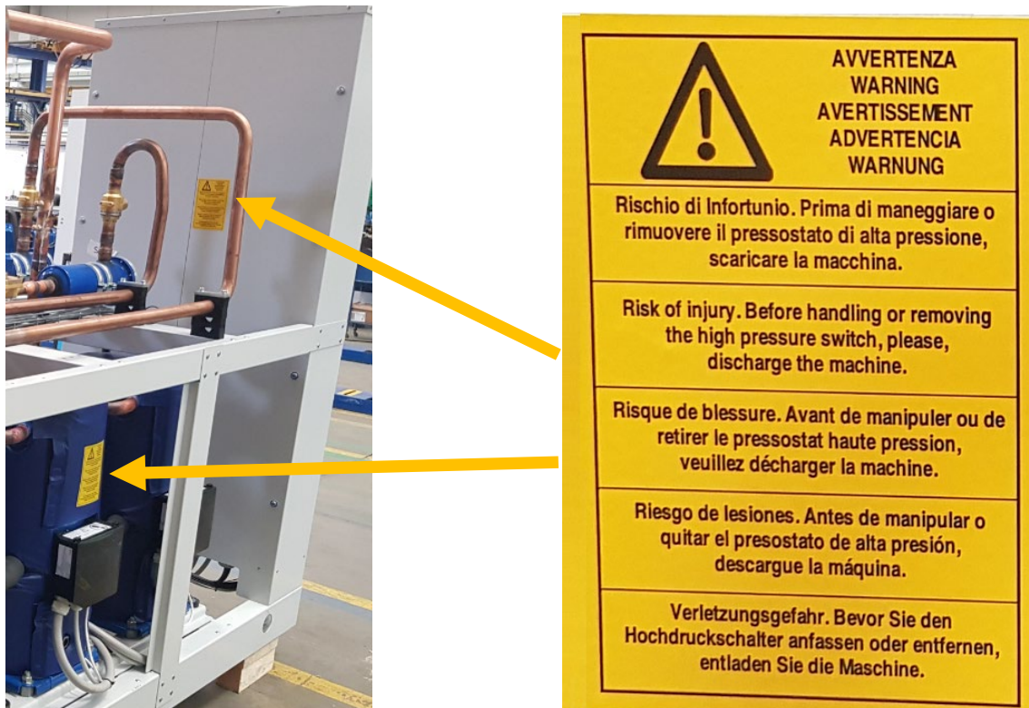
Figure 1 – Indicative position of the signs warning about the necessity of replacing the high pressure switches with the unit void of refrigerant
